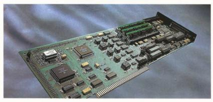
This exciting new board combines all the features of GVP's best products to date. It consists of a 68030 Accelerator board and a full SCSI hard disk controller. It is even possible to mount a slimline hard disk directly onto the card. As a 68030 processor is being used, the 9MB memory limit of the Amiga is no longer a problem, and large amounts of memory can be added using GVP's special design of 32-bit Simm
